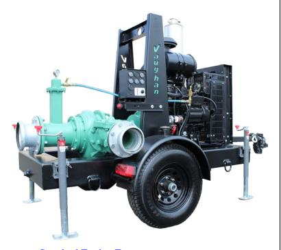
Standard Engine Features: Safety shutdown switches for low oil pressure and high temperature. Instrument panel with temperature, oil pressure, amp-meter, hour-meter and tachometer gauges. Muffler with rain cap. Engine to pump coupling: SAE3 housing with 10" rubber disc drive.
